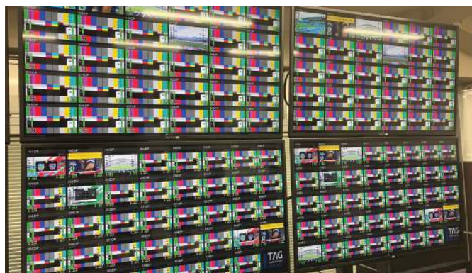
MCM-9000's penalty box function displays an alert (yellow bar) on streams where an error is detected.
